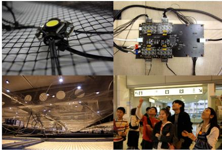
Figure 3. LED on a plastic net, LED controller board, display in situ, and viewers at the airport (from top left to bottom right).
