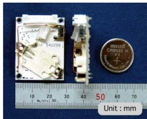
**Figure 3.** "S-Node" RFID nodes (LED nodes) and a CR2032 button lithium battery.
