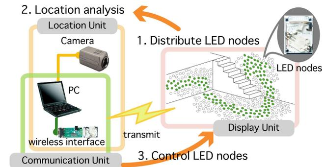
**Figure 2.** System diagram of the Particle Display System.
